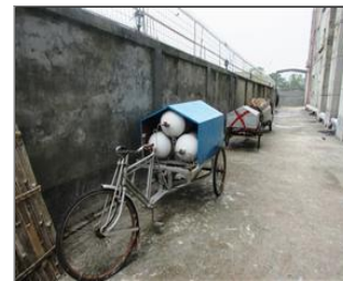
Photo of non-conformity NG- Gas Cylinder not protected.JPG
